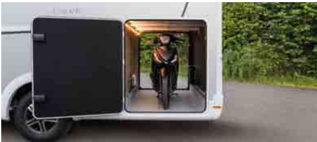
+ Room for everything: High rear garages with 250 kg loading capacity and accessible from both sides. An LED strip provides the necessary illumination.
