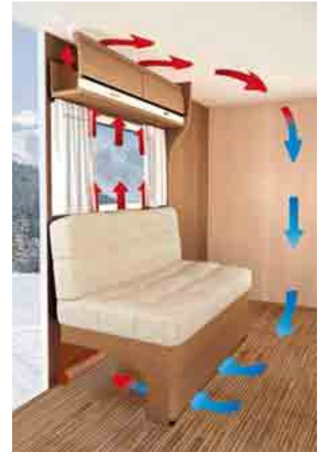
+ Good indoor climate: The air ventilation behind the overhead lockers avoids condensation
