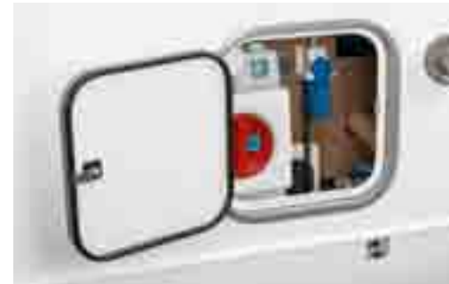
+ Service access for filling and cleaning the fresh water tank, the 230 volt socket
