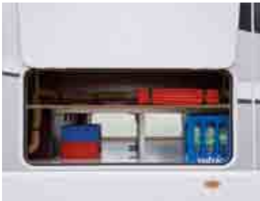
+ Frost-protected: 40 cm high, heated double floor with lots of storage space
