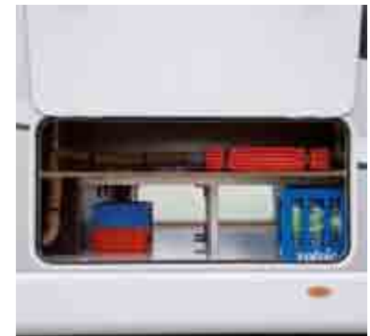
+ Frost-protected: 40 cm high, heated double floor with lots of storage space
